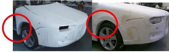
Fig.20: Prototype of the bumper before (left) and after the adjustments
