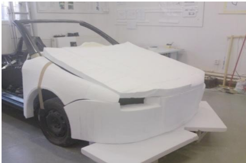
Fig. 7: Model fabrication and preparation of laminating molds (scale 1:1)
