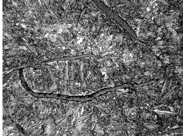
Fig. 5 Microstructure of the material after marquenching and tempering, etch. pikric acid, 500x
