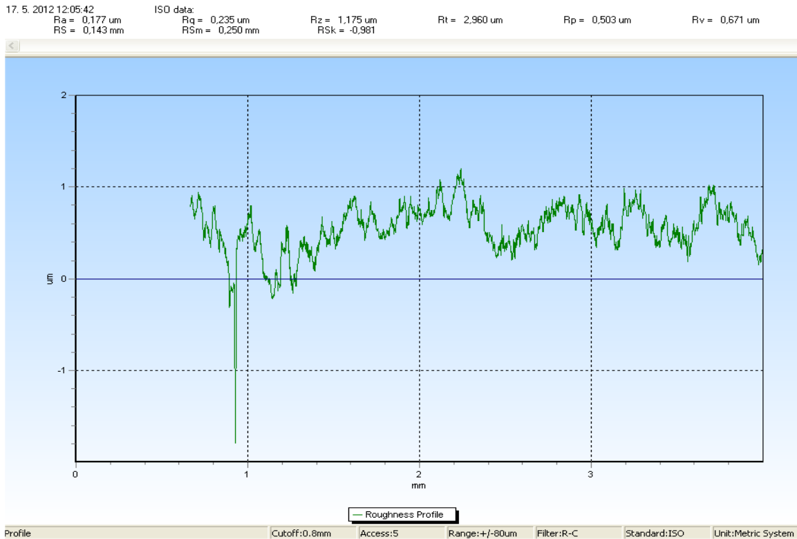
Fig.6 Graph of surface profile of polyamide bushing after the test
