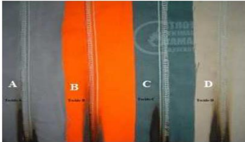
Figure 4 – Bodies of Proof with Thread 2 after the Flammability Test
