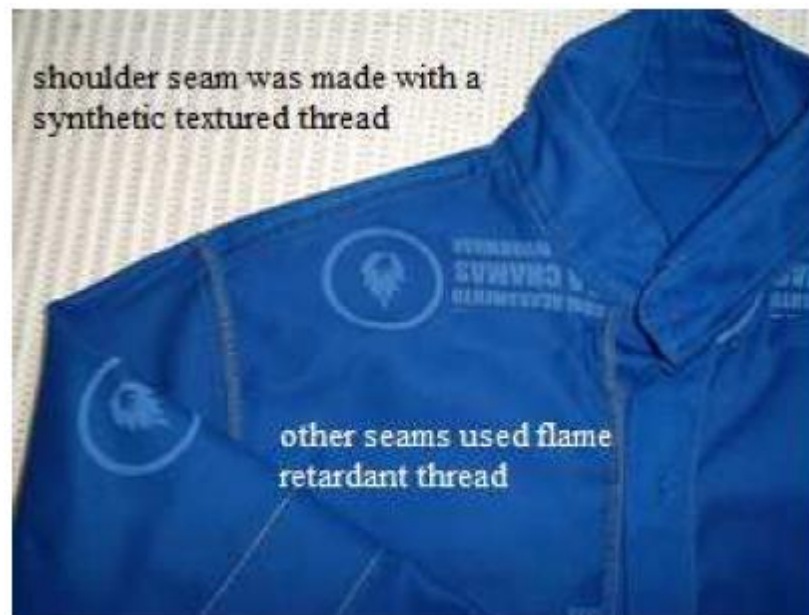
Figure 11 – Inside Out of a Shirt in Flame-Retardant Fabric Sewn with Two Different Kinds of Threads: Thread Flameretardant Fiber and Synthetic Textured Filament Thread
