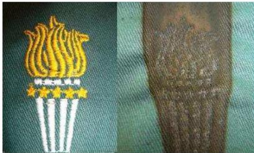
Figure 2 – Embroidery Before and After the Flammability Trial
