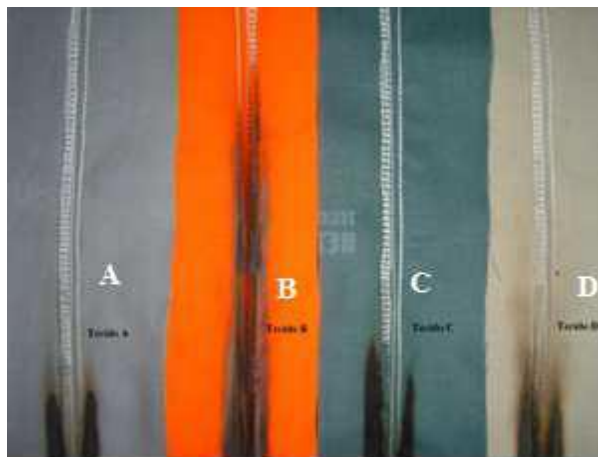
Figure 5 – Bodies of Proof with Thread 3 after the Flammability Test
