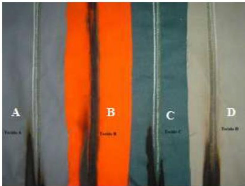
Figure 6 – Bodies of Proof with Thread 4 and Thread 5 (Textured Filament) After the Trial
