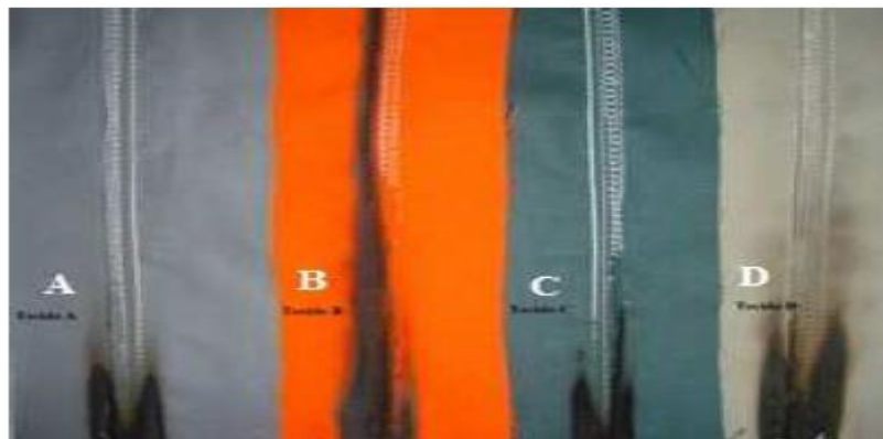
Figure 3 – Bodies of Proof with Thread 1 after the Flammability Test
