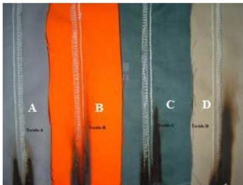
Figure 7 – Bodies of Proof with Thread 2 in Loopers and Thread 4 in Needles after the Flammability Trial
