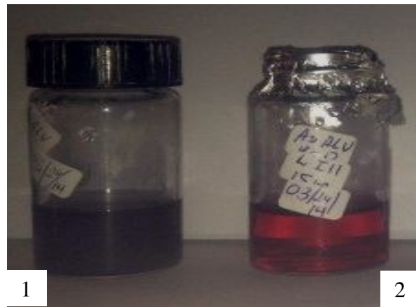
Fig.6. Visual appearance of the biosynthesized AgNP nanosolution: (1) after laser illumination, (2) before laser illumination
