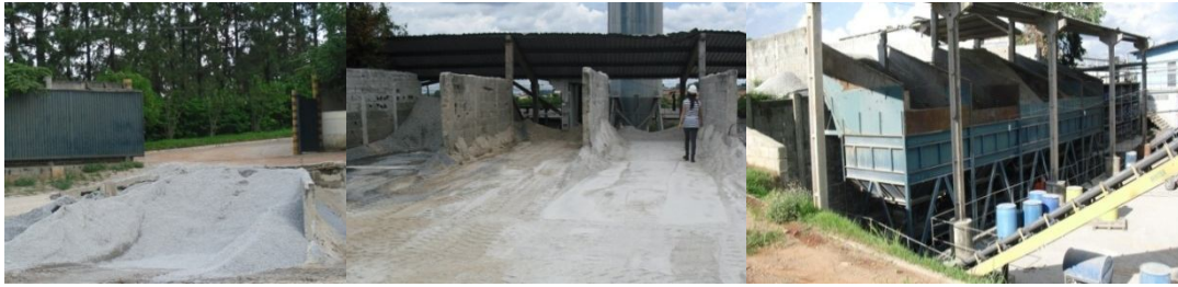
Figure 2 - (a) Drying Bays (“Rest”), (b) Storage Bays, and (c) Measurement Stations
