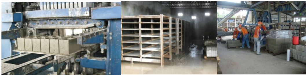
Figure 3 - (a) Exit of Blocks from Blocopac 900 (b) Drying Chamber, and, (c) Block Palletizing
